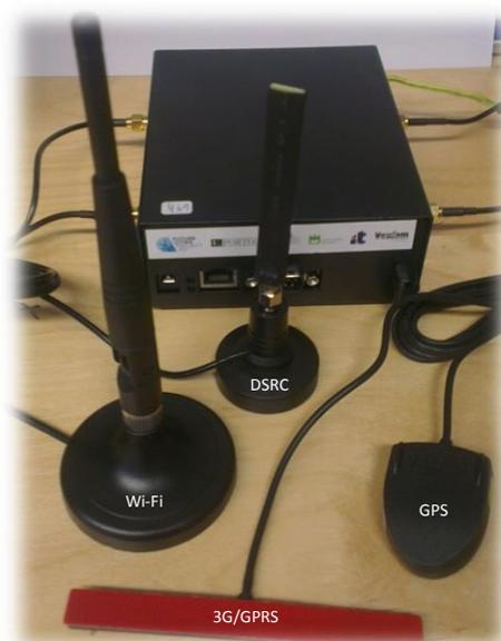
**Figure 3.1** – On-board unit and external antennas (Wi-Fi, DSRC, GPS and 3G/GPRS).
